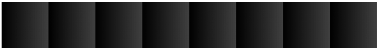
Fig. 81: Test Image Seven for 8 bit Output Modes Generated with a Raw or Enhanced Raw Line Acquisition Mode (Raw - Line A First and Enhanced Raw - Line A First as an Example) on a Camera with 4096 Pixels Per Line
