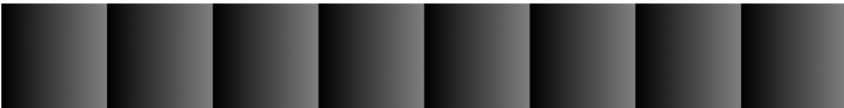
Fig. 84: Test Image Eight for 8 bit Output Modes, Generated with a Raw or Enhanced Raw Line Acquisition Mode on a Camera with 4096 Pixels Per Line
